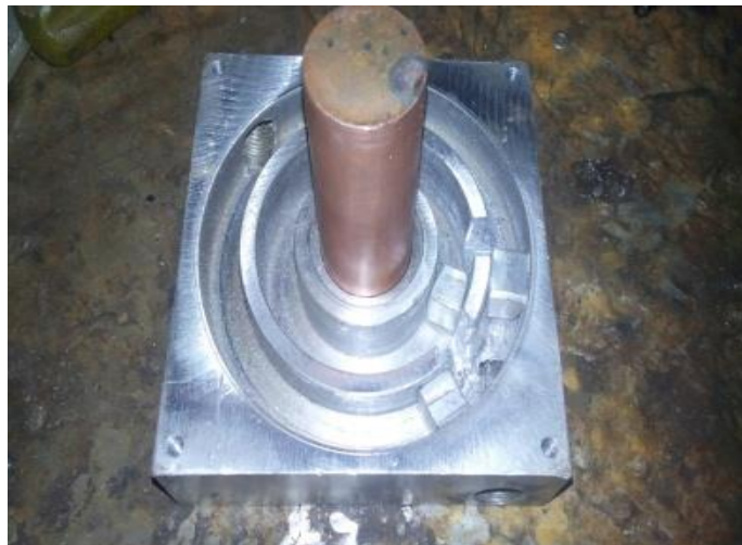
Fig- 2: Hybrid vortex aluminium plate with sintered copper heat pipe
