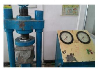
Fig.3. Flexural Strength test in UTM
