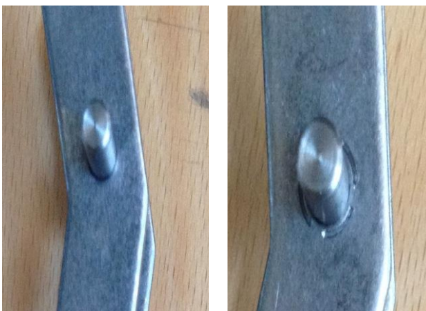
Fig 6.7 Schematic diagram of Double Lever caulking.
