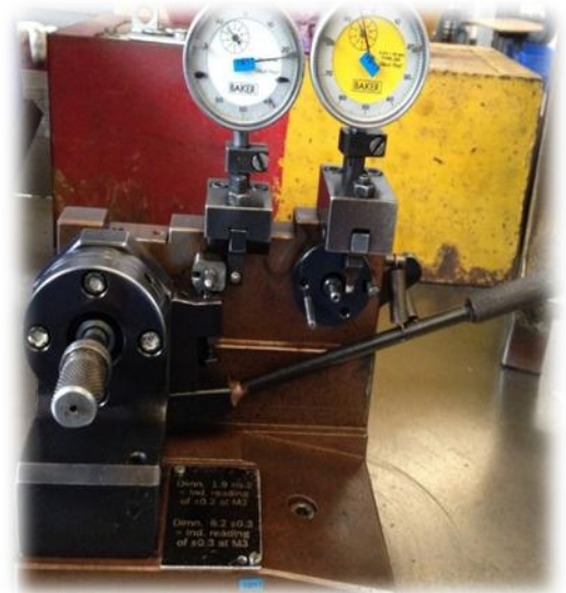
Fig 6.4 The gauge used for checking straightness of floating lever.
