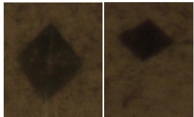
FIG 2 Indent on hardness sample Solution Treated and 40%Room temperature rolling respectively.
