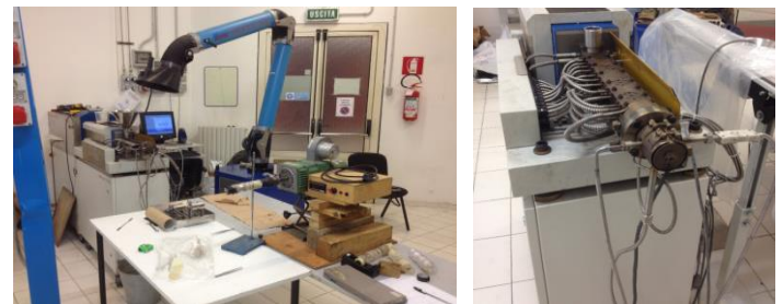
Fig. 2 Spinning units (a) external view of extruder with heating units (b) filament production units.
