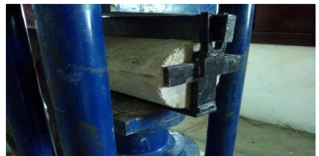
Fig.3 Testing of cylinders for Split tensile strength
