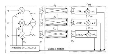
Fig -1: Block diagram of the multiple independent SU-MIMO beamforming system.
