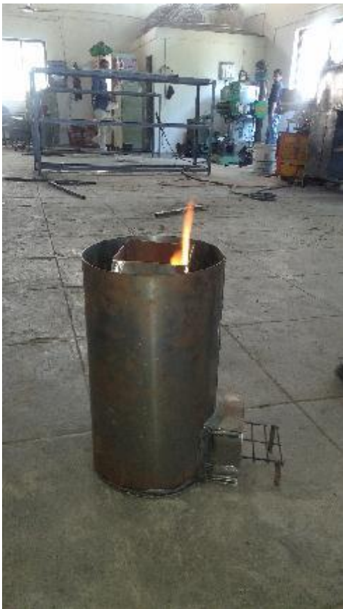
Fig-2: TESTING PROCEDURE FOR THERMAL EFFICIENCY TEST
