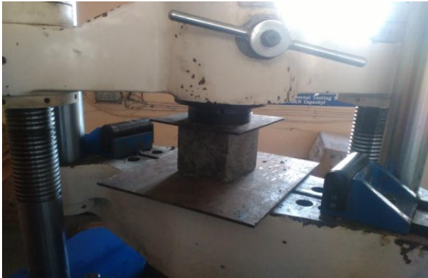
Fig no. 2. Compressive strength test on concrete
