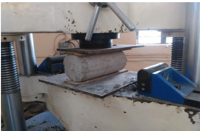
Fig no. 3. Split tensile strength test on concrete
