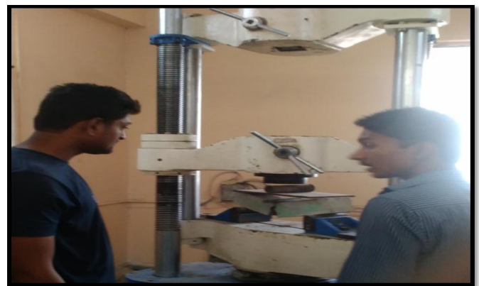
Fig no. 4. Flexural strength test on concrete
