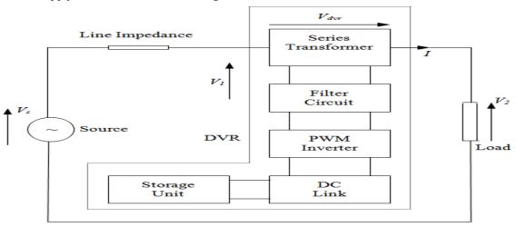
Fig. (1) A Simplified Block Diagram of Dynamic Voltage Restorer (DVR)
