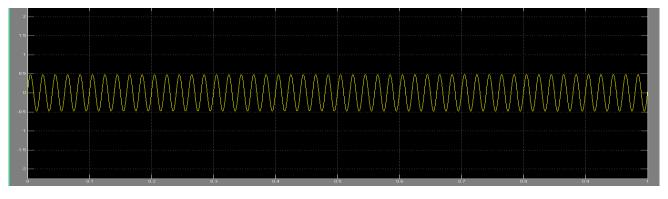
Fig.(4d): Load voltage of phase-A during single-phase fault
