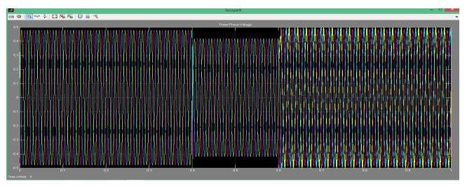
Fig.(4b): Load voltage during three-phase fault
