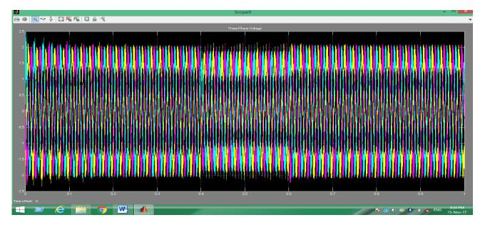
Fig.(4c): Load voltage after the DVR operation on three-phase fault
