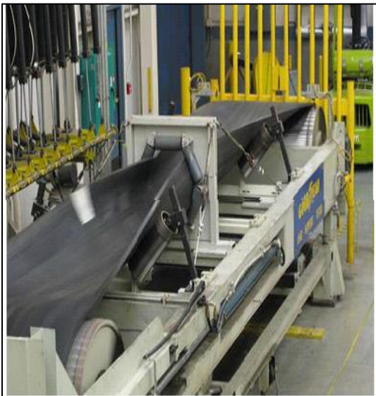
Figure 3. Pipe belt transition test
