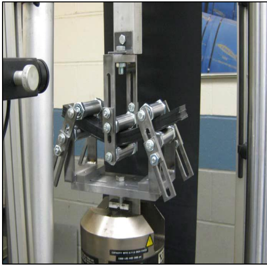
Figure 2. 3 point bending stiffness test.
