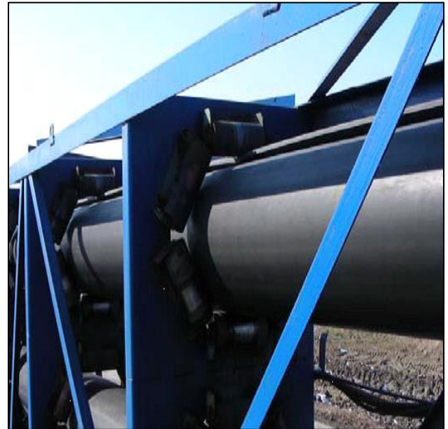
Figure 6. 400mm diameter ST1100 Low Rolling Resistance Pipe Belt.
