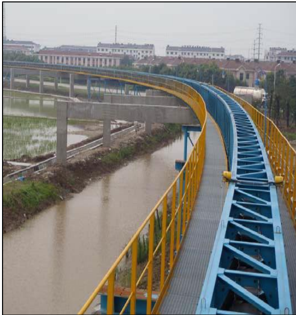
Figure 8. 350mm diameter ST2000 EPDM heat resistant pipe belt, with material temperature 180°C.
