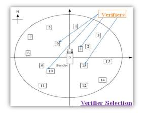
Fig -7: Verifier Selection for Compound Method
