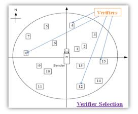
Fig -6: Verifier Selection for Most-Distributed Method
