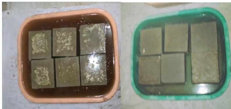
Figure.7 Specimens in MgSO 4 & NaCl
