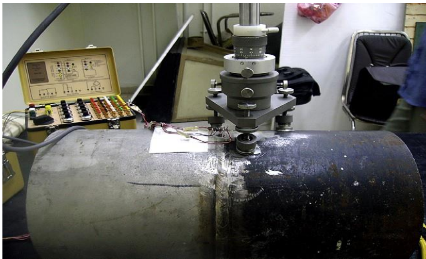
Fig. 8. Experimental setup of Hole drilling method
