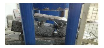
Fig.-1 Flexural beam test of specimen
