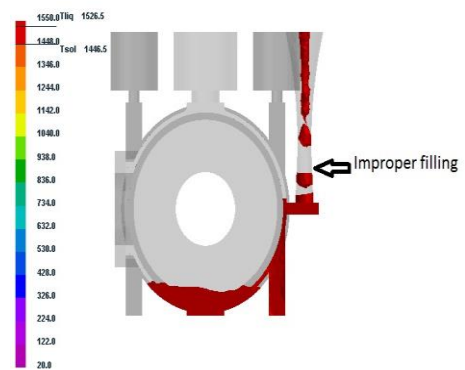
Fig: Improper filling in step 10
