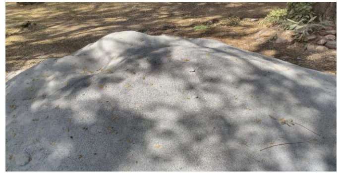
Fig-2 Crushed fine aggregate used for replacement of fine aggregate
