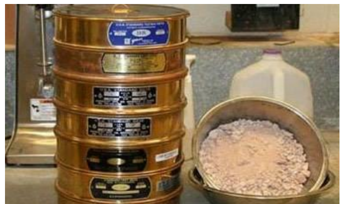
Fig -1: Apparatus of sieve analysis of Fine Aggregate
