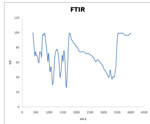
Fig 2(c) FTIR Spectrum of ZTS
