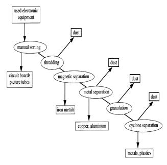
Fig 4 Generic e-waste treatment flow diagram
