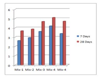
In the chart it is seen that when Glass powder & Coconut shell content is increased there is an increase in flexural strength will be increased with a maximum at 15%. However when the Glass powder & Coconut shell content is increased beyond this value (20%) a downward slope observed. This must be due to cluster of Waste Glass Powder which can crust the binding and strength formation in concrete.
