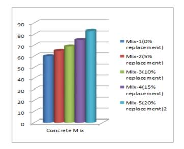
From the table it is observed that the desired slump value is obtained for Mix 5 at water cement ratio = 0.43 is maximum. Hence we fix it as the design ratio. Mix 2 and 3 yielded very low slump values which was very close to Mix-1(conventional) may be either due to inadequate paste available for binding the mix or due to improper mixing procedure.
