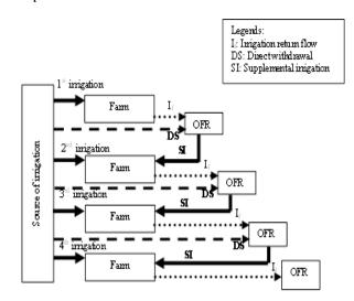
Fig. 1: Flow diagram showing the source of water to OFR and its utilizations
