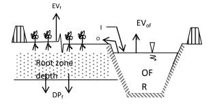
Fig. 3.b Cross-section of lined OFR with flow details
