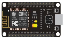
Fig 4 – Wi-Fi Module ESP 8266
