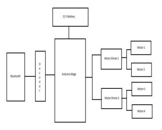
Fig 7 – Block Diagram of WSR
