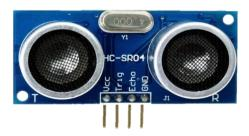
Fig 2 – Ultrasonic sensor HC-SR04
