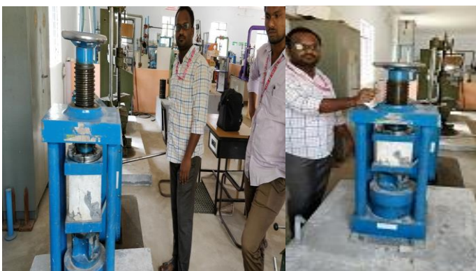
Fig 2: Shows compressive strength test for cubes
