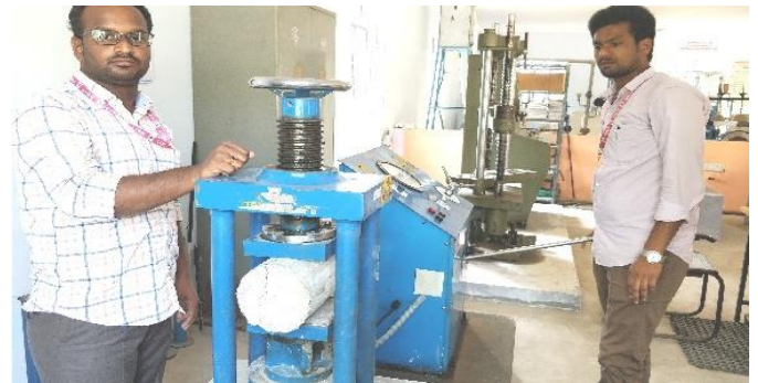
Fig 3: Shows split tensile strength test for cylinders
