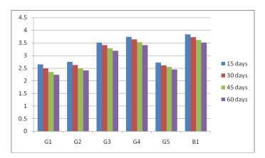
Fig- 6: Flexural strength of GPC and OPC Specimens after immersing in acid
