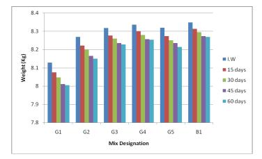
Fig-11: Weight of GPC and OPC Specimens after immersing in acid
