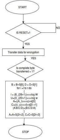
Figure 8. Flow chart for encryption in RC6
