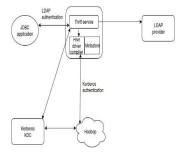
Figure 6 Security In Hadoop Using Kerberos
