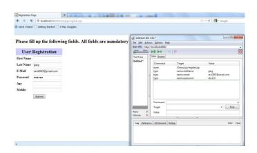
**Fig -5**: Screen for entering the value of field E-Mail & corresponding record in selenium.
