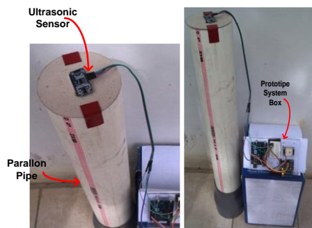
Fig- 8: The Construction of Water Level Detection Device
