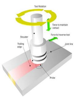
FSW is a solid-state joining process that creates high-quality, high-strength joints with low distortion and is capable of fabricating either butt or lap joints, in a wide range of material thicknesses and lengths.
