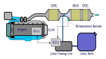
Fig2: Selective Catalytic Reduction process
