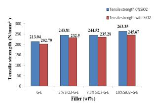
Fig 5: Comparison of Tensile strength behavior of with and without silica powder (SiO<sub>2</sub>)
