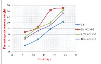
Fig 8: Water absorption of composites during 24days of immersion in distilled water
