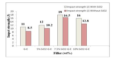
Fig 7: impact test behavior with and without silica powder (SiO<sub>2</sub>)
