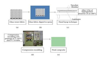
Fig 2: Schematic Representation of composite fabrication process
