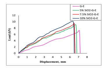
Fig 4: Load vs. displacement graph for SiO<sub>2</sub>G-E composites
