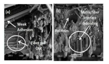
Fig 11: SEM micrographs of tensile fractured surfaces of Unfilled G-E composites
