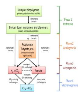
Fig 2. Stages of production of biogas[1-2]
