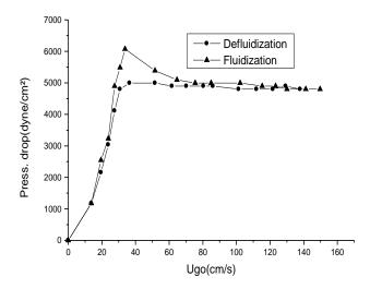
**Plot -1**: Effect of superficial gas velocity on pressure drop In bed with cone angle of 20.5°
