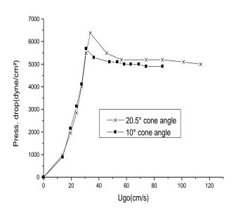
Plot -4: Effect of cone angle of conical bed with stagnant height 5 cm on fluidization with coarse particles
