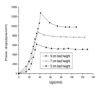
**Plot -3**: Effect of stagnant bed height of the conical bed  $(\theta = 20.5^{\circ})$  on fluidization with coarse particles
