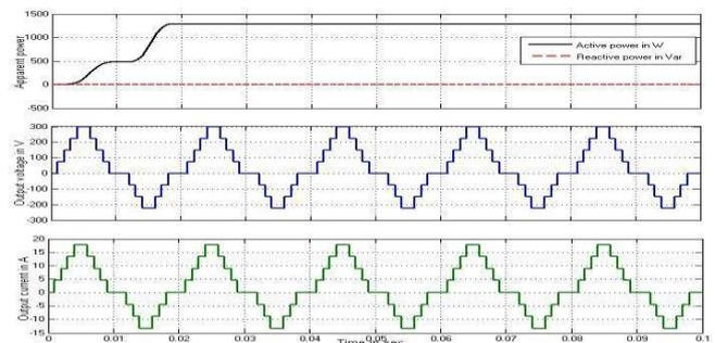
Figure 4.5 waveforms of nine level inverter (one switch fail)
