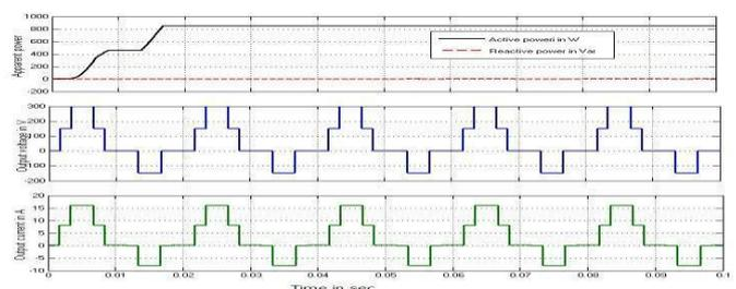
Figure 2.5 Output waveforms when switch failed to turn on
