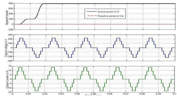
Figure 4.4 waveforms of nine level inverter (one battery disconnected)
