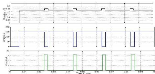
Figure 2.3 power loss across switch
