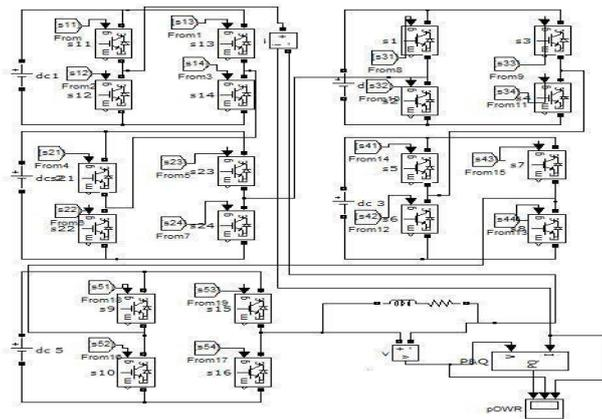
Figure 5.1 Simulation of nine level inverter
