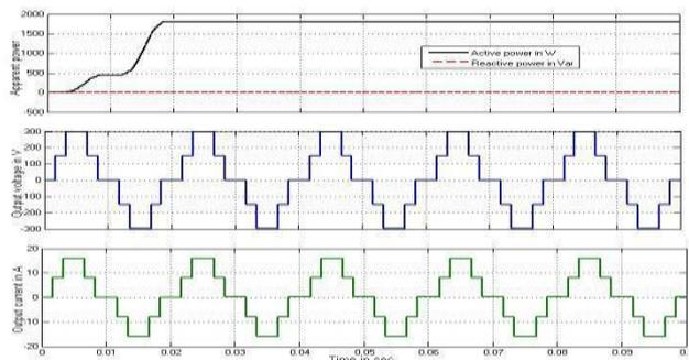
Figure 2.2 output waveforms of Five level inverter at u.p.f.
