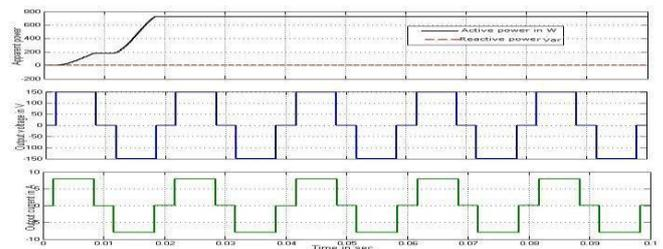
Figure 2.4 waveforms when one battery source disconnected
