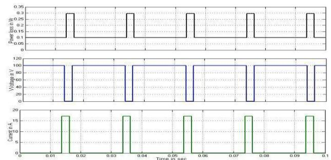
Figure 3.3 power loss across switch
