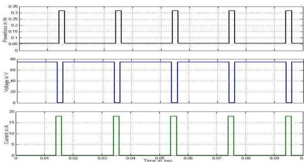
Figure 4.3 switching transients across the switch
