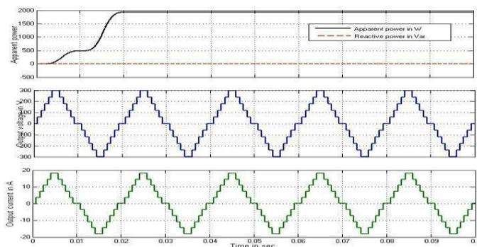
Figure 5.2 Output waveforms of eleven level inverter at u.p.f.
