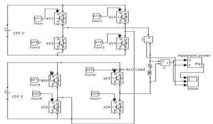
Figure 2.1 simulation of five level inverter
