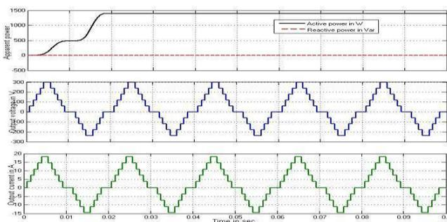
Figure 5.5 waveforms of eleven level inverter (one switch fail)
