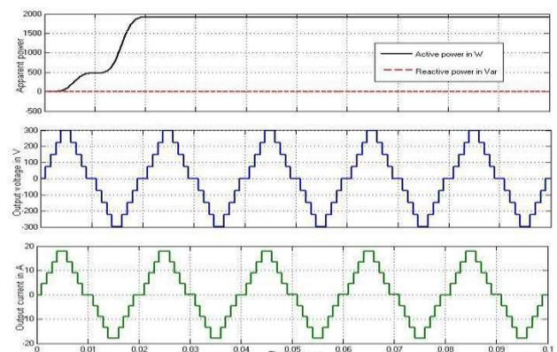
Figure 4.2 output waveforms of Nine level inverter at u.p.f.
