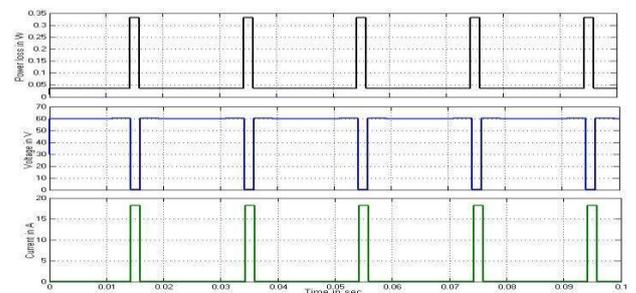
Figure 5.3 Voltage transients across switch
