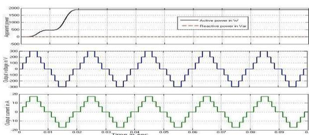
Figure 3.2 output waveforms of Seven level inverter at u.p.f.
