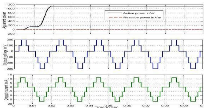
Figure 3.5 Waveforms of seven level inverter (one switch fail)
