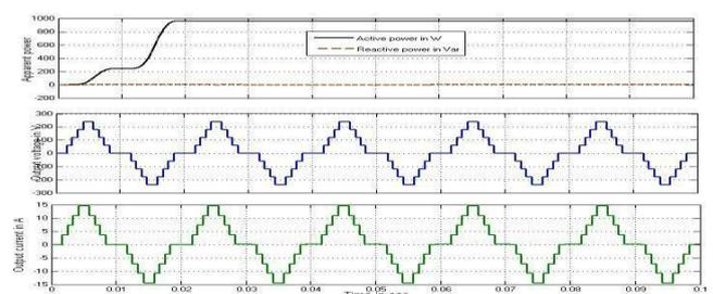
Figure 5.4 Waveforms of eleven level inverter (one battery disconnected)
