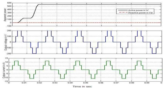
Figure 3.4 waveforms when one battery source disconnected
