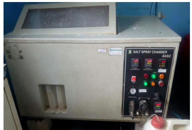
Figure 4.1: Salt spray Testing Equipment
