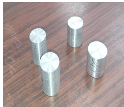
Figure 4.2: Salt spray Testing specimen.
