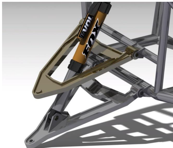
Figure 1. 3D Rendered CAD model of Double wishbone suspension system
