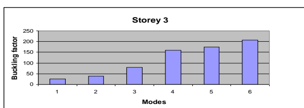
Fig- 6 Buckling modes v/s Buckling factor
