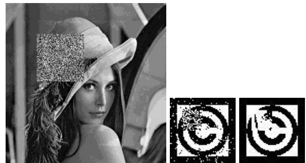
Fig-4: Region based tempering and corresponding recovered watermarks in DCT and DWT domain respectively
