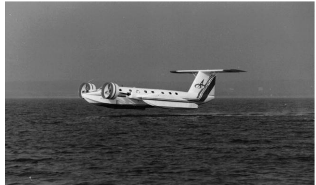
Fig -2: A WIG Aircraft Flying Over Water (Courtesy of WIG Vehicle Development Center of Chinese Academy of Science Technology Development).
