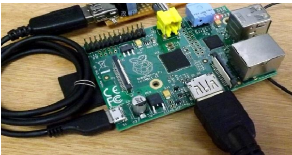
Fig-7.4 Raspberry pi connected with UART
