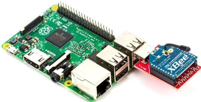
Fig-7.3: XBee is configured with raspberry p Step5: In base station stored the all data, the client can visit directly to the base station.
