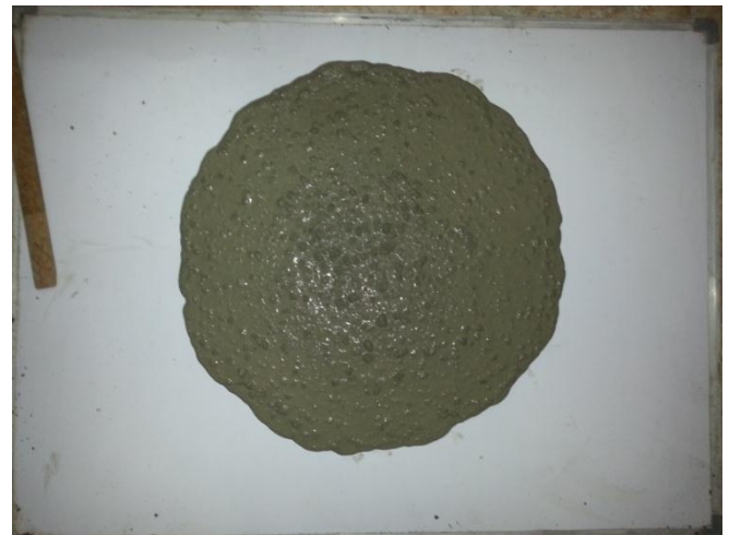
Fig.1. Slump Flow Test
