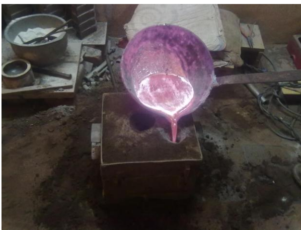
Fig-3: Pouring of molten metal into mould cavity
