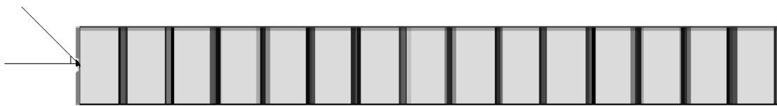
Figure 1: Schematic representation of a one-dimensional periodic medium. The coordinate system and light rays refracting and propagating through a stack are shown. The angle of incidence is designated by \theta_i . Refractive indices of alternating regions and an ambient medium are n_\alpha, n_\beta ( n_\alpha < n_\beta ) and n , respectively. Thicknesses of alternating regions are t_\alpha and t_\beta . T = t_\alpha + t_\beta is a period.
