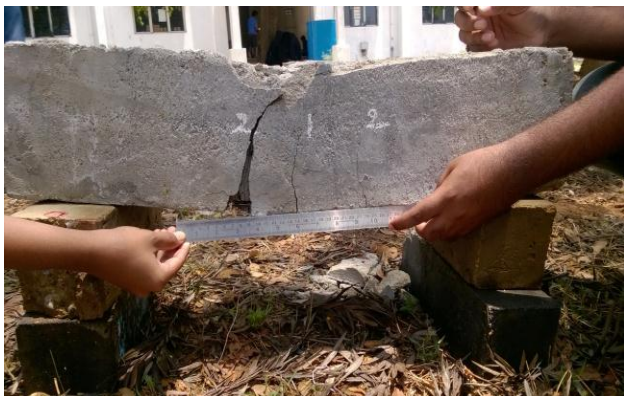
Fig -8: Cracking pattern of jacketed beam by 1 layer mesh at orientation of 45 degree reinforced ferrocement with connectors
