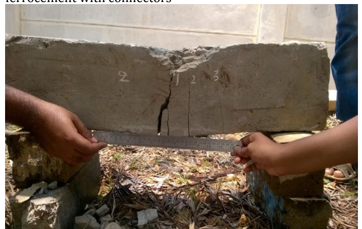
Fig -9: Cracking pattern of jacketed beam by 2 layer mesh at orientation of 45 degree reinforced ferrocement with connectors
