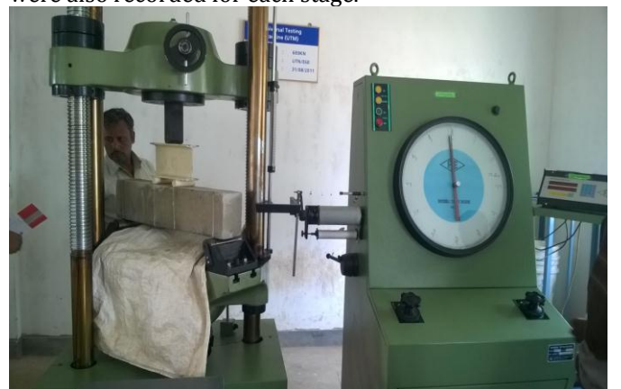
Fig - 5: Universal Testing Machine with flexural test setup
