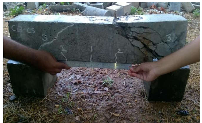
Fig -7: Cracking pattern of Control beam with corrosion steel
