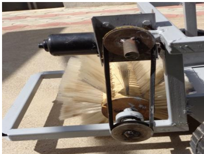
Fig -6: Horizontal Rolling Brush with driven belt drive
