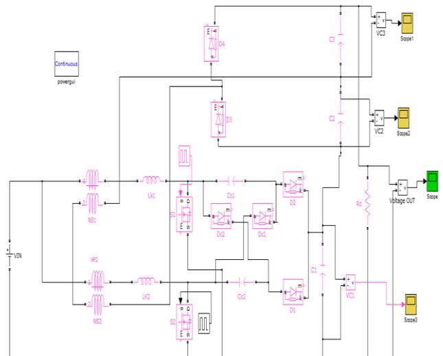
**Fig -8:** Simulink model of the High Step up Converter
