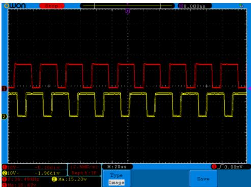
Fig -13: Switching pulses of the Converter
