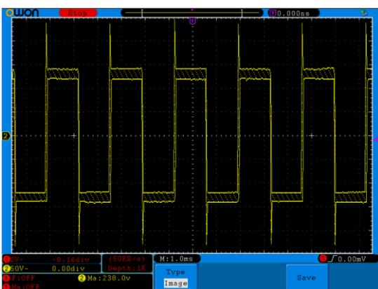
Fig -15: Output voltage from the Inverter
