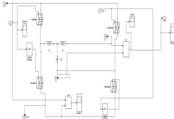
Fig -9: Simulink model of the Inverter
