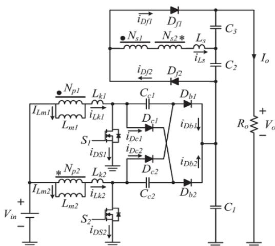
Fig -3: Equivalent circuit of High step up converter
