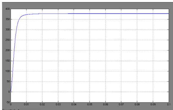
Fig -10: Output voltage of the High Step up Converter
