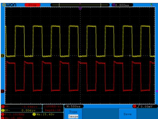
Fig -14: Switching pulses of the Inverter
