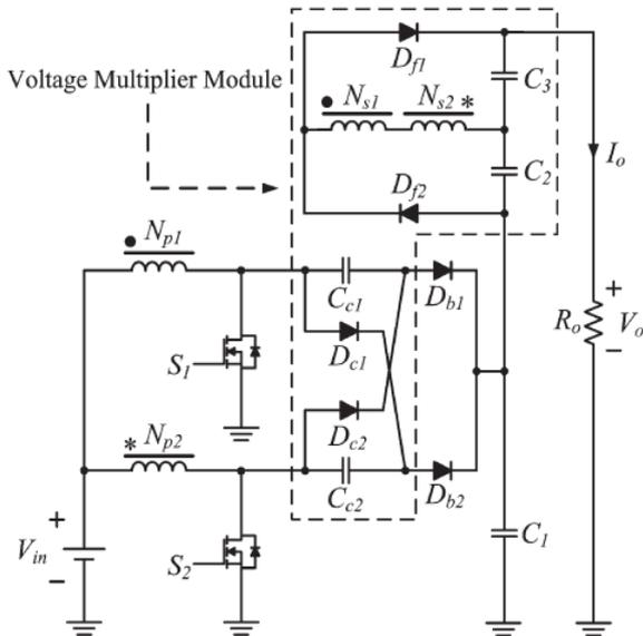
Fig -2: High step up converter with voltage multiplier
