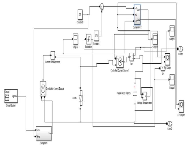
Fig -4: Simulink model of the PV Panel
