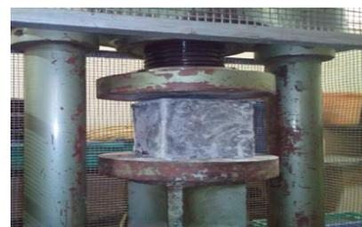
**Fig-1:** Compression Test
