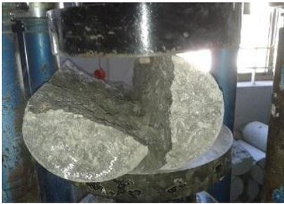
Fig-3: Tensile Test
