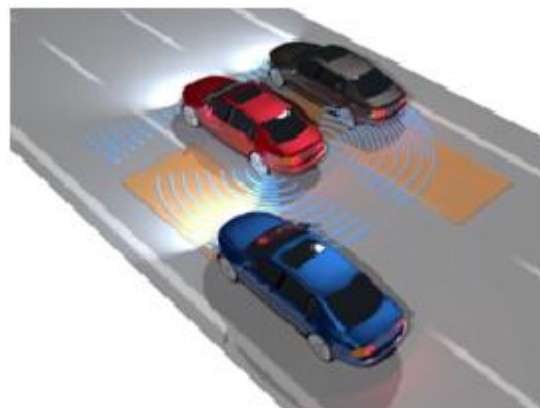
Figure 4: Blue car is in the blind spot of red car's driver. The blue arcs depict the sensor range of the red car's sensors. The orange rectangles depict the critical zone which should be supervised.
