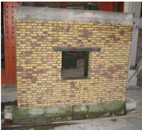
Fig -1: Unreinforced masonry wall
