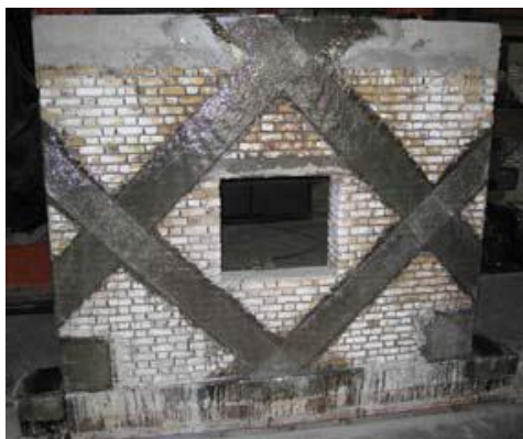
Fig -2 : GFRP strengthened wall
