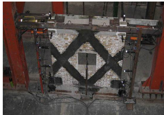
Fig -3: Cyclic load test setup
