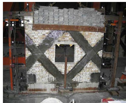
Fig -4 : Vertical load test setup
