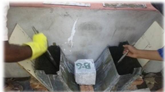
Fig -8: Compacting the Mix
