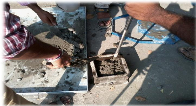
Fig -5: Compacting the concrete in to cube shape
