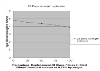
**Graph -2: 1.00% & of Replacement of Glass Fibers in Steel by weight for cylinder.**
